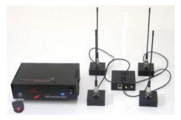
Doppler DF: Using a beam or body-shadowing has the disadvantage that is takes at least a few seconds to get a reading. If the interference is happening in short bursts, you need faster readings. One popular option is the so-called "Doppler DF". This uses four antennas mounted in a square on the roof of the vehicle (or other metal ground plane) and a control box that rapidly (at an audio rate) switches between the four antennas in sequence. Each time the antenna is
